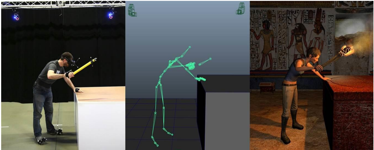
Fig.2: From Real to Virtual. How the system interprets motion capture data and renders it in a 3D environment.
