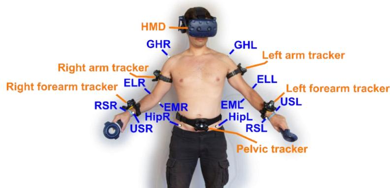
Figure 1: Fully equipped subject with the HMD, a controller in each hand and the trackers (orange) strapped to pelvis, upper arms, and forearms. The image also shows the Vicon's optical markers placed on anatomical landmarks (blue).
