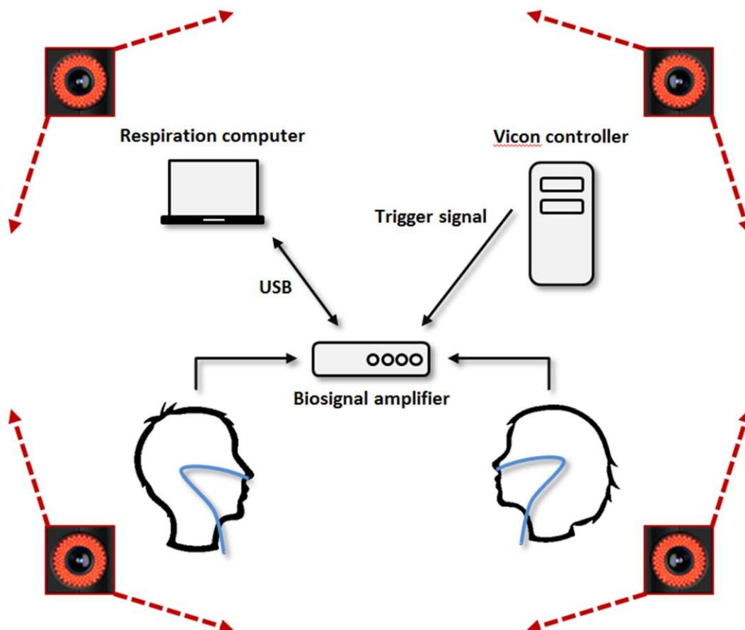
**Figure 1: Hardware setup:** the respiration data of the two participants was passed through a biosignal amplifier to the respiration computer. The Vicon controller received body motion data from the participants. The two systems were synchronized using a digital signal sent from the Vicon controller to the respiration computer through the digital input channel of the biosignal amplifier.
