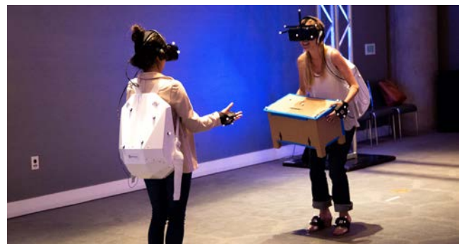
Figure 2. Two users interacting with a physical object: in the virtual world the users can see an Egyptian chest, whereas it is a simple cardboard box in the real world.
