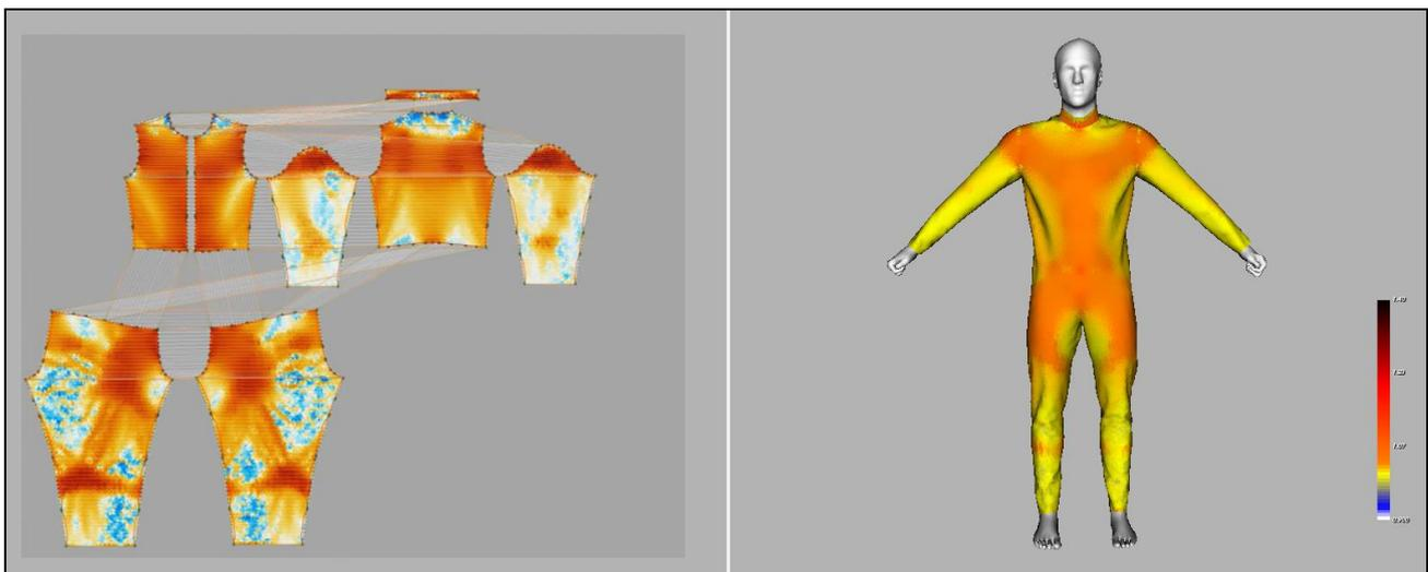
Figure 4: Motion fitting data in 2D shown on the flat pattern (left) and on the 3D cloth (right).
