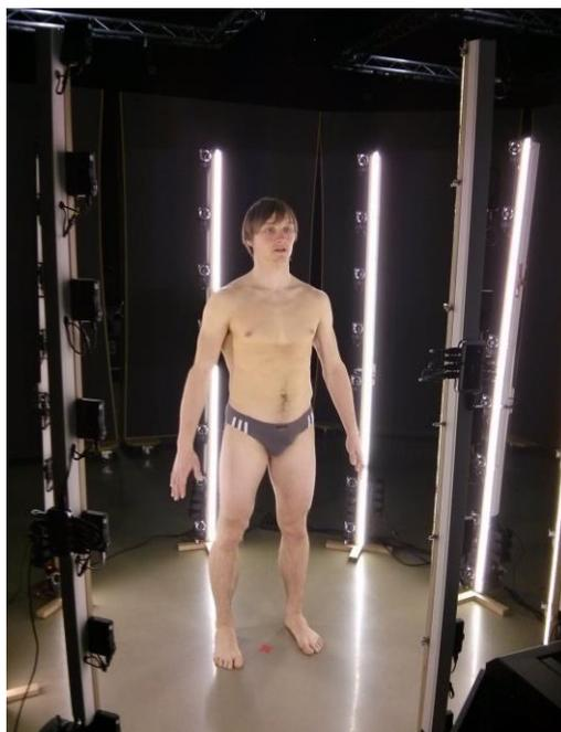
Figure 1: Photogrammetric 3D body scanner with subject standing in A-pose.
