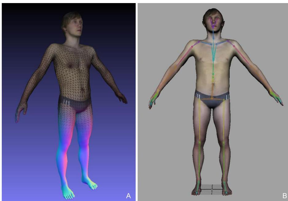
Figure 2: 3D body mesh generated from the body scanner: A) after post-processing, B) with underlying skeleton used to drive animation.
