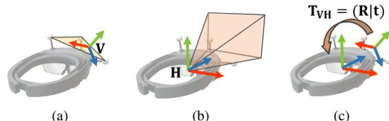
Figure 1: (a) Coordinate system arbitrarily defined by optical markers rigidly attached to the headset. (b) Coordinate system of the headset aligned with camera projection. (c) The calibration determines the rigid transformation – rotation  $\mathbf{R}$  and translation  $\mathbf{t}$  – that aligns the tracked coordinate system to the headset’s coordinate system.
